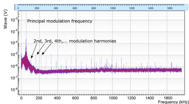
**Figure 5.** Pump signal's Fourier transform measured with the Oscilloscope of LabOne user interface. The plot shows a prominent peak at the principal modulation frequency 54 kHz, while the 2<sup>nd</sup>, 3<sup>rd</sup>, 4<sup>th</sup>, ... harmonics are about 80 dB below the amplitude of the main peak.
