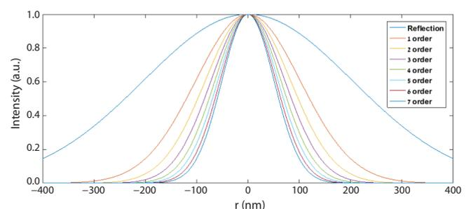
**Figure 1.** Simulated profiles of the effective PSF on the lateral ( $r$ ) axis calculated from the PSF and the  $n$ -th order of the pump intensity distribution. The blue curve represents a probe reflection scan, while the other curves correspond to the  $n$ -th order of TR.
