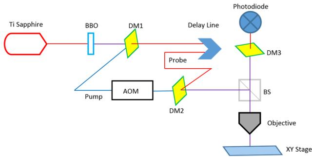
**Figure 2.** Optical setup comprising dichroic mirrors (DM), an acousto-optic modulator (AOM), a beam splitter (BS), and a photodiode.
