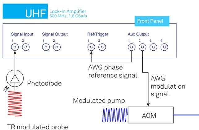
**Figure 4.** Electrical setup used to generate the pump beam modulation and to measure the photodiode signal. The AWG output on Auxiliary Output 1 is connected to the AOM driver. The photodiode signal is measured with the UHF-Lock-in Amplifier. The Ref/Trigger connectors are used to phase-lock the UHF-AWG with the lock-in amplifier.
