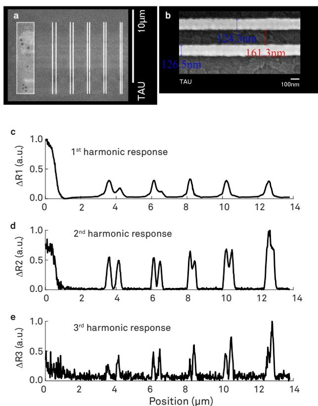
**Figure 6.** Super-resolution line imaging of gold on sapphire nanostructures. The sample consists of gold double lines, 125 nm wide, with decreasing gaps of 370, 270, 160, 160, and 120 nm, respectively. (a) High-resolution scanning electron microscope (HR-SEM) image of the sample. (b) HR-SEM zoom on one of the 160 nm gap double lines. (c-e) Line scan with a 0.95 NA objective using the 1<sup>st</sup> (c), 2<sup>nd</sup> (d), and 3<sup>rd</sup> (e) harmonic of the modulation.
