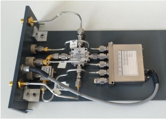
Figure 3. Photo of the up-conversion board.
