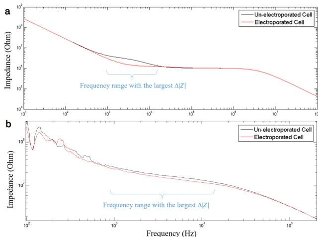
**Figure 2.** (a) Simulated cell impedance as a function of frequency for an unexposed (black curve) and electroporated (red curve) cell. The region of significant change in  $\Delta|Z|$  is shown from 1 to 10 kHz. (b) Frequency sweep from Zurich measuring changes in cell impedance under the same conditions and parameters as that of the simulation.
