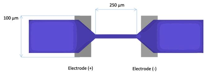
**Figure 3.** Microfluidic device with channel diameter channel constriction is  $250 \times 25 \times 10 \mu\text{m}^3$ , electrodes are  $100 \mu\text{m}$  wide separated by  $300 \mu\text{m}$ .
