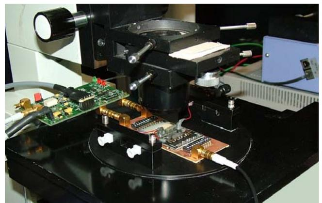
Figure 1. Microfluidic setup using electrical impedance spectroscopy.
