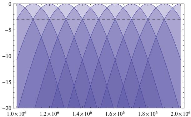
Figure 1. Linear frequency sweep from 1 MHz to 2 MHz: the dashed line indicates the minus 3 dB level
