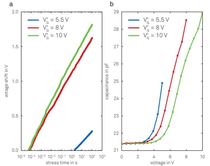
**Figure 6.** C-OTF measurement results including its dependence on the sweep voltage extrema  $V'_G$ . (a) Flatband voltage shift during the stress time (b) CV curve.
