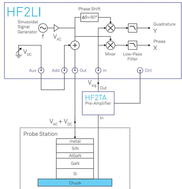
**Figure 4.** Schematic diagram of the experimental setup including the lock-in HF2LI, the pre-amplifier HF2TA and the probe station as well as the HF2LI electronics using phase sensitive detection in order to get phase X and quadrature Y.
