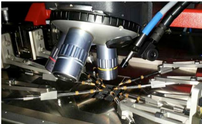
**Figure 3.** Needle probe station with mounted sample.
