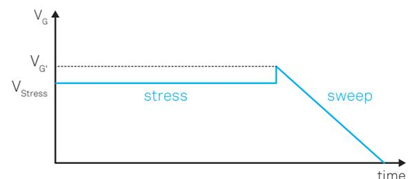
**Figure 1.** Schematic diagram of the capacitance on-the-fly method, in which a device is stressed for some time at a certain stress voltage  $V_{\text{Stress}}$  followed by afterwards a sweep of the gate voltage starting from  $V_G$  and going to zero is applied.
