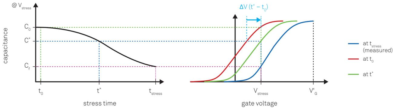
**Figure 2.** Time dependent capacitance during a constant stress voltage corresponds to a shift to the right in the capacitance voltage curve (indicated by the orange arrow).
