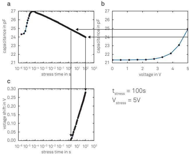
**Figure 5.** (a) Capacitance transient during the stress voltage  $V_{\text{stress}}$ . (b) CV curve obtained from the stress voltage extrema  $V'_G$  downwards. (c) Calculated flatband voltage shift using the capacitance transient and the CV curve.
