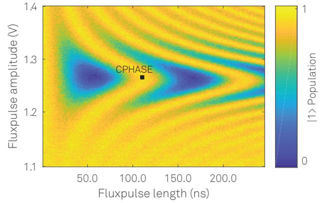
**Figure 4.** Chevron-Pattern of the CPHASE gate. A first  $\pi$ -pulse on both qubits is used to bring the system in the  $|11\rangle$  state and then a flux pulse with variable amplitude and length is applied, followed by the readout of qubit 2.
