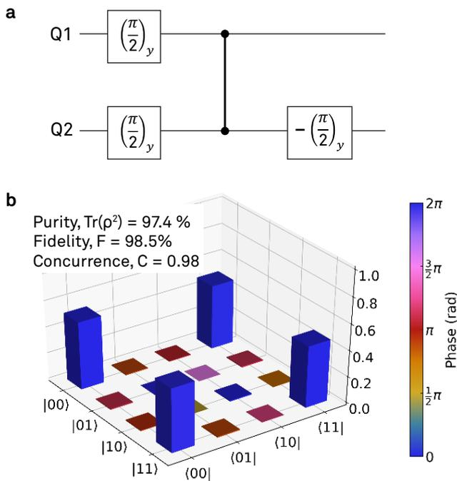
**Figure 5.** Bell state tomography: (a) Pulse Sequence for preparing the Bell state. The state was prepared with the aid of a CPHASE gate, illustrated by a vertical line. (b) Density matrix measured by state tomography. The obtained raw data was fitted with a Maximum-Likelihood estimation.
