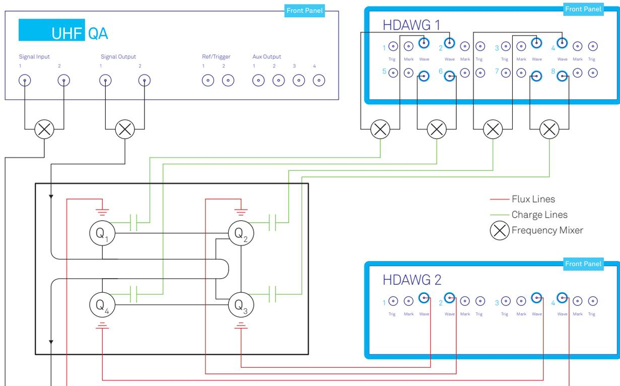
**Figure 2.** Simplified sketch of the 4-qubit experiment. Qubit readout is carried out by the UHFQA, qubit state manipulation by HDAWG 1 and qubit-qubit coupling is activated by HDAWG 2. For simplicity the local-oscillators, microwave amplifiers, filters and attenuators are not included in this sketch; see [4] for further details.
