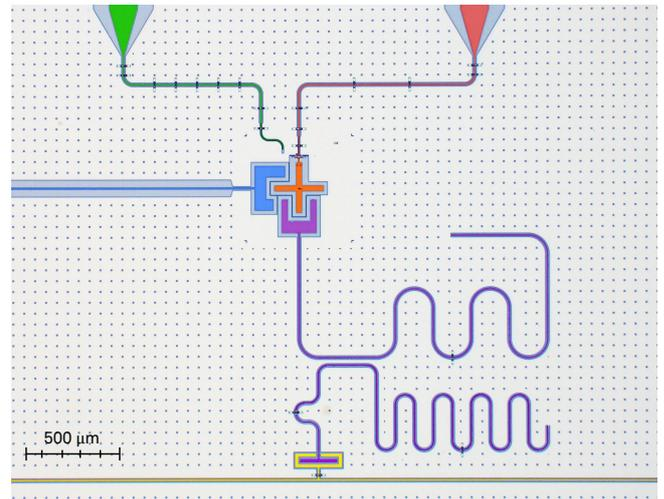
**Figure 1.** Colored microscope picture of a qubit unit cell: charge-line (green), flux-line (red), qubit island (orange), coupling resonator (blue), readout circuitry with Purcell-filter (violet) and feed-line (yellow). The chip substrate is Silicon with Niobium as a superconducting metal layer. [3]
