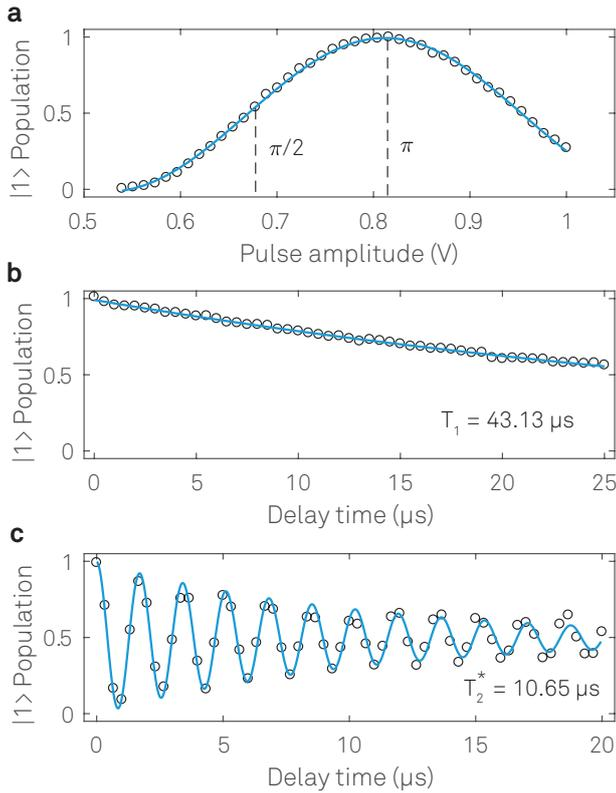
**Figure 3.** Single qubit characterizations: (a) Rabi-oscillation, (b) Qubit lifetime  $T_1$  measurement and (c) Ramsey fringe measurement to extract  $T_2^*$ .
