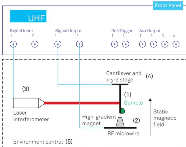
**Figure 1.** Schematic of basic wiring of a UHFLI within an MRFM setup. Signal Output 1 drives the cantilever and provides active feedback, e.g. for Q control, Signal Output 2 is used to generate the RF signal. Signal Input 1 reads the the signal from the interferometer.
