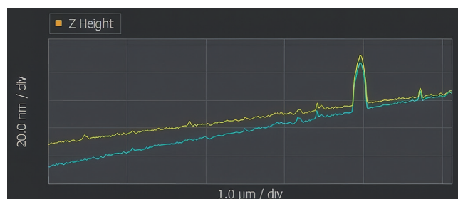
Figure 7. Determining Z-drift. By observing the Z Height raw data, a drift of roughly 20 nm is present between the beginning of the forward trace and the end of the backward trace. If this drift exceeds the lift height, the tip will crash into the surface while scanning. While operation at a 60 nm lift height would be possible at 20 nm drift, measurement data will be influenced by the effective non-constant lift height. Thus, it is strongly recommended to wait until the drift has settled.
