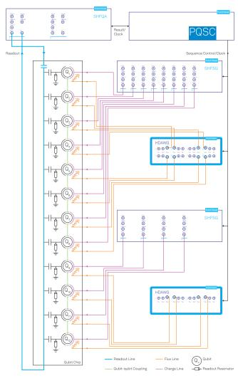
Example setup showing how 12 superconducting qubits can be controlled and read out in a QCCS system. An SHFSG-8 and SHFSG-4 provide the microwave control signals for qubit gate operations, while the HDAWG-8 and HDAWG-4 provide flux pulses for tuning the qubit frequencies. By frequency multiplexing the readout, all 12 qubits can be read out using a single channel of the SHFQA-2. The data and measurement timing are synchronized across the instruments by the QHub.
