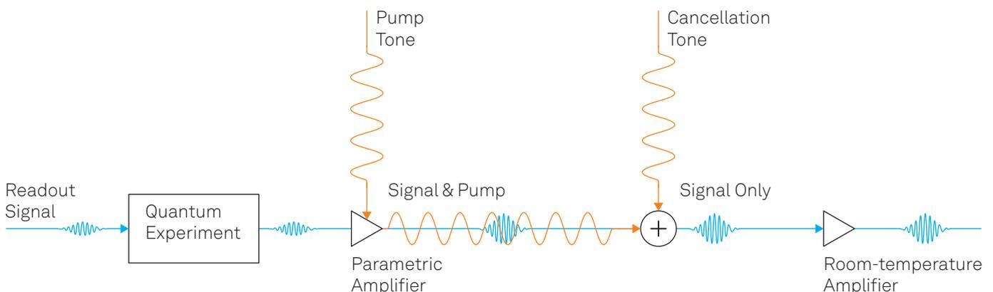
Representation of a readout chain for a Quantum Experiment, featuring a Parametric Amplifier to amplify the Readout Signal. The Pump Tone driving the amplifier is generated and cancelled by the SHFPPC, leaving only the desired measurement signal.
