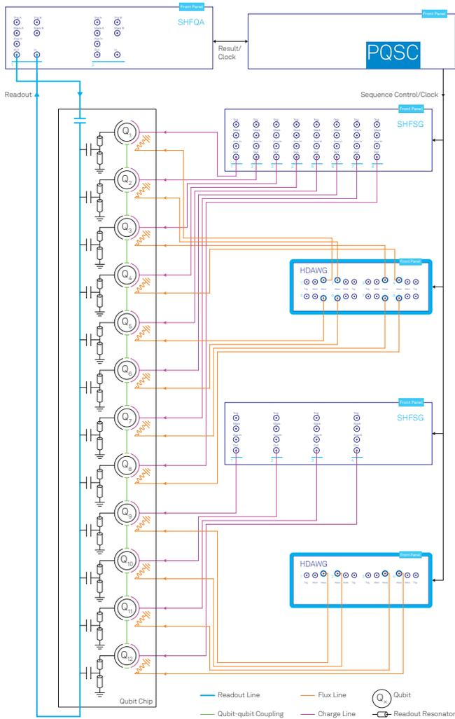
Example setup showing how 12 superconducting qubits can be controlled and read out in a QCCS system. An SHFSG-8 and SHFSG-4 provide the microwave control signals for qubit gate operations, while the HDAWG-8 and HDAWG-4 provide flux pulses for tuning the qubit frequencies. By frequency multiplexing the readout, all 12 qubits can be read out using a single channel of the SHFQA-2. The data and measurement timing are synchronized across the instruments by the PQSC.
