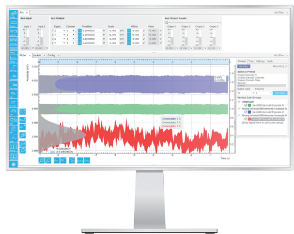
Figure 15. The LabOne® user interface of Zurich Instruments' lock-in amplifiers uses the latest web browser technology. The instruments can be controlled from multiple browser sessions on various PCs, tablets, etc. at the same time. Every signal analysis and control tool has a dedicated tab. Some of the functionality is intuitively displayed in form of block diagrams.
