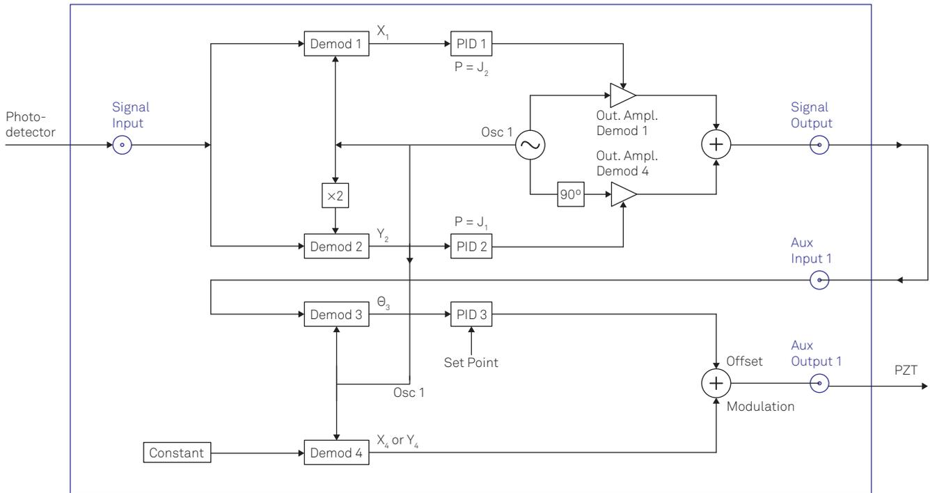
**Figure 4.** Detailed description of the instrument configuration to be implemented using the LabOne user interface. In total, 4 demodulators (Demods) of the instruments are required. Two PID controllers are used as proportionate functions to apply the Bessel coefficients. The third PID controller is used to drive the offset signal controlling the mirror displacement.
