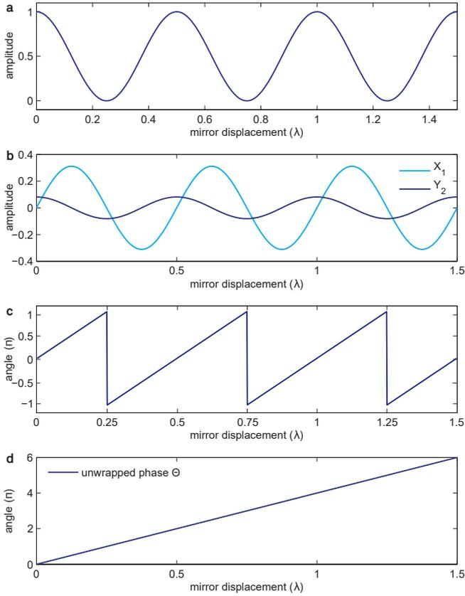
**Figure 2.** (a) shows the sinusoidal signal detected by the photodetector over the relative displacement between mirrors 1 and 2. (b) shows the signals  $X_1$  and  $Y_2$  demodulated at  $\Omega$  and  $2\Omega$ . (c) shows the phase angle between the normalized  $X_1$  and  $Y_2$  components given in Equation 5. (d) shows the unwrapped version of the same phase in (c) used by the PID controller to drive the PZT.
