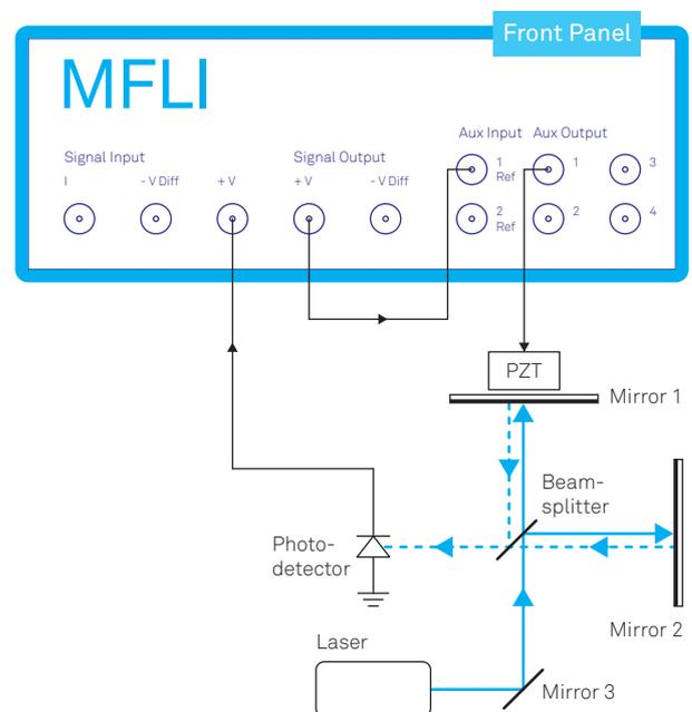
**Figure 1.** Michelson-Morley interferometer actively stabilized by a closed-loop system using the Zurich Instruments MFLI Lock-in Amplifier. The Auxiliary Output provides both a modulating signal and a controlling offset for the piezo electric transducer (PZT). The external loop-back from the Signal Output to the Auxiliary Input is required to generate the linearized and continuous error signal for PID control (see text).
