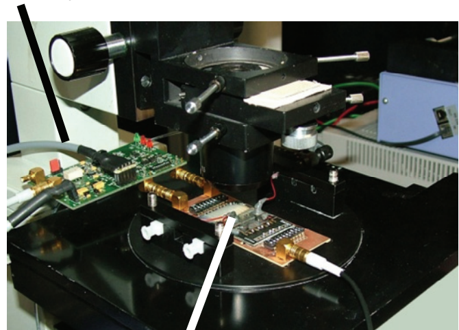
Figure 4: Picture of the measurement setup with microscope, microchip holder, and preamplifier.
